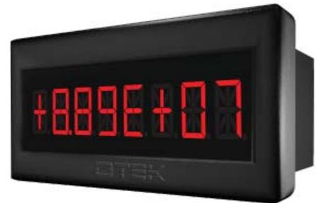
**Up/Down Timer (Option A):** Just like the Up/Down Counter (Option 1), but instead of using external pulses to count, the UPM uses its internal programmable time base to increment/subtract its count. Default is one (1) second, range is 1 μs to 10 seconds.
