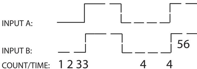
**Elapsed Time (Option C):** Depending on the model selected (number of characters/digits), you can display/control events in days, hours, minutes, seconds, mS, and μS (D:365, H:24, M:60, S:60, μS:000,000 for a 15 digit model(s) or 5 digits for the smallest package (-L). Use the relays, O.C.T. or analog output to control your process by setting limits/alarms (usually 00:00:00).
