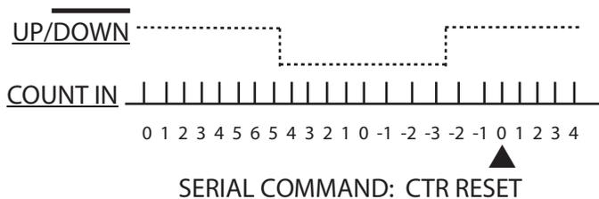
**3.1 Zero Datum:** (also see "Quadrature" and "Up/Down" Counter) This single pulse/revolution is produced by rotary encoders to indicate 0° and it is used by the UPM to zero its display and start counting up or down in a degree fashion with degrees, minutes, second, and milliseconds of rotation determined by the resolution of your encoder. For linear measurements, use command "LIN." For rotational, use the command "ROT."
