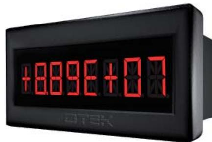
**Up/Down Timer (Option A):** Just like the Up/Down Counter (Option 1), but instead of using external pulses to count, the UPM uses its internal programmable time base to increment/subtract its count. Default is one (1) second, range is 1 μs to 10 seconds.
